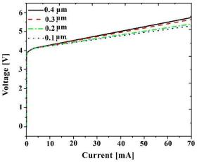
Fig. 9. V-I curves for LDs with different p-AlGaN thicknesses.
