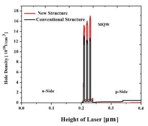
Fig. 14. Hole densities of the conventional and the optimized new quadruple asymmetric waveguide LDs.
