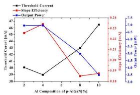
Fig. 4. Threshold current, output power and slope efficiency of LDswith various compositions of Al in the Al<sub>x</sub>Ga<sub>1-x</sub>N p-cladding layer.
