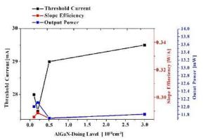
Fig. 10. Threshold current, output power and slope efficiency of LDs with different p-AlGaN doping levels.
