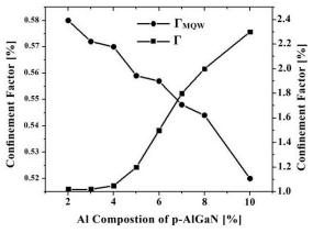
Fig. 3.  $\Gamma_{MQW}$  and  $\Gamma$  as an Al composition function in the Al<sub>x</sub>Ga<sub>1-x</sub>N p-cladding layer.
