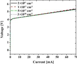
Fig. 11. V-I curves for LDs with different p-AlGaN doping levels.
