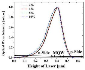
Fig. 5. Optical field distributions for LDs with various compositions of Al in the Al<sub>x</sub>Ga<sub>1-x</sub>N p-cladding layer.
