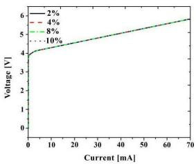
Fig. 6. V-I curves for LDs with different compositions of Al in the  $Al_xGa_{1-x}N$  p-cladding layer.
