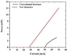
Fig. 12. L-I curves for the conventional and the optimized new structure LDs
