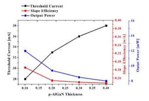
Fig. 8. Threshold current, output power and slope efficiency of LDs with different p-AlGaN thicknesses.
