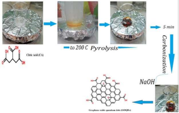
Fig. 1. The preparation process of GOQDs.
