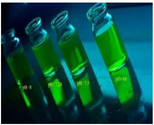
Fig. **6.** Photographs of GOQDs under UV light ( $\lambda = 360nm$ ) in various pH values.
