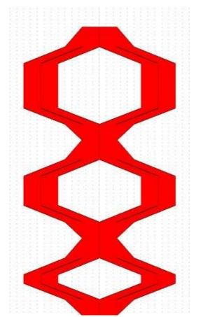
Fig. 3. Design of a Triple ring resonator waveguide.
