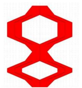
Fig. 2. Design of a double ring resonator waveguide.
