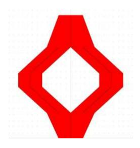
Fig. 1. Design of a single ring resonator waveguide.
