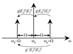
**Fig.1.** Energy flow between the three waves, pump, Stokes, and anti-Stokes, due to Raman scattering. g and g' are the parallel Raman gain coefficients at the frequency detuning  $\Omega$  and  $2\Omega$ , respectively.
