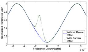
**Fig. 5** Normalized parametric gain for various Stokes waves detuned from the pump frequency. Dotted curve is for a case where Raman scattering is included, and dashed curve is for a case where only SMI is considered. Fiber length and pump power are 100m and 1 W, respectively.
