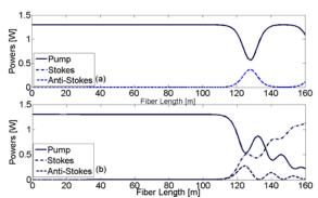
Fig.2 the evolution of pump, Stokes, and anti-Stokes along the PCF due to SMI: a) without Raman Scattering, b) with Raman Scattering. The input pump power is 1.3 W. In Fig. 2(a), the curves of Stokes and anti-Stokes are coincided.
