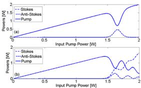
Fig. 3 The output power of the pump, Stokes, and anti-Stokes as a function of input pump power due to SMI: a) without Raman scattering, b) with Raman scattering. The fiber length is fixed at 100m. In Fig. 3(a), the curves of Stokes and anti-Stokes are coincided.
