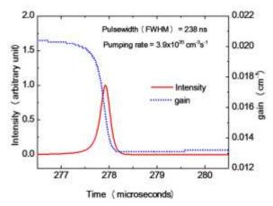
Fig. 10. The calculated laser intensity and optical gain of the Q-switched Ce:Nd:YAG laser with  $E_p = 0.7 J$  similar to conditions of Fig. 6.
