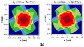
Fig. 9. The calculated values of: a) absorbed power versus the shared area of laser rod and, b) pumping profile across the cross-section of laser rod for Nd:YAG and Ce:Nd:YAG active medium at  $\lambda_p = 592 \ nm$  and  $\lambda_p = 460 \ nm$ , respectively.
