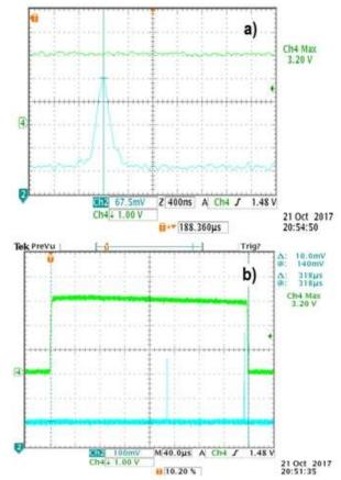
Fig. 5. a) Time behavior of the first Q-switched pulse with  $E_p = 1.2\ J$ , b) the position of the first and second Q-switched pulses are respectively 188 and 312 microseconds after the rising edge of LEDs current pulse.
