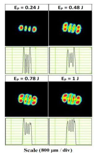
Fig. 8. The Ce:Nd:YAG laser free-running mode profiles along their major axis of symmetry for the different values of pump energy.
