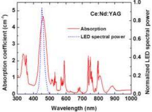
Fig. 1. Absorption spectrum of Ce:Nd:YAG crystal with 0.1 and 1.0 atomic percent concentration of Ce<sup>3+</sup> and Nd<sup>3+</sup>, respectively and normalized spectral power of the blue LED with peak emission at 460 nm [2].
