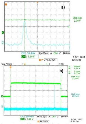
Fig. 4. a) Typical laser time behavior of a 240 ns single Q-switched pulse slightly above threshold  $E_p = 0.7 \ J$ , b) the position of the Q-switched pulse is 278 microseconds after the rising edge of the LEDs current pulse.
