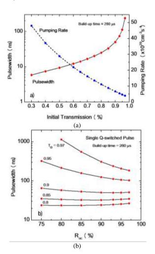
Fig. 11. a) Calculated laser pulse-width and required pumping rate versus initial transmission  $T_0$  of the Cr:YAG passive QS, b) pulse-width versus reflectivity of output coupler for different values of  $T_0$ . For all cases the pulse build up time is  $t_b = 280 \ \mu s$
