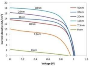
Fig. 3. The JV characteristics of the representative J-V curves for the PSC devices with various thicknesses of the C70 layer as ETL.
