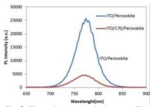
Fig. **5.** The steady state photoluminescence (PL) measurements of the ITO/perovskite and ITO/C70(10nm)/perovskite films
