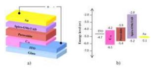
Fig. 1 a) Planar PSC device architecture with C70 as ETL, b) Energy level diagram of PSC with a conventional device configuration.
