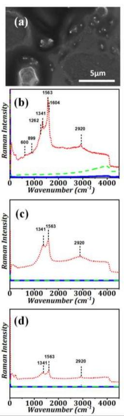
Fig. 3. (a) FESEM image of 10<sup>-?</sup> M phenylalanine amino acid on the SERS substrate. Raman spectra of (blue-solid curves) the SERS substrate, (greendash curves) phenylalanine on glass substrates; and SERS spectra of (red-dot curves) phenylalanine on the SERS substrates. The concentrations of
