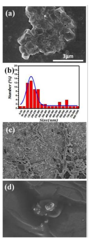
Fig. 4. FESEM images of (a) the SERS substrate. (b) The size distribution of silver larger particles and silver nanoparticles. FESEM images of blood
