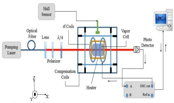
Fig. 1. Earth's magnetic field measurement setup. Laser beam was transported by an optical fiber to the magnetometer, where it was collimated and circularly polarized. Then, it passed the cell which was heated by a nonmagnetic heater, and finally the beam entered a photo-detector. The output of the photo-detector was fed to a lock-in amplifier and the lock-in controlled the frequency of RF coils. At the same time the output of photo-detector was read by a computer for data analysis.
