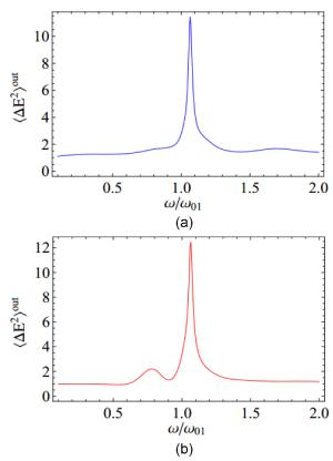
Fig. 2. Quadrature variance of Eq. (10) for an incident squeezed light with the squeezing strength  $\rho=0.2$  and the phase  $\phi_{\rm p}=2\phi_{\rm LO}-2$ . Here, the thickness of the loss and gain slabs is l=500nm. The Homodyne detection is placed at (a) the right and (b) the left hand-sides of the  ${\cal PT}$ -symmetric bilayer structure.
