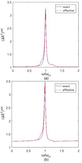
Fig. 3. Comparison of the quadrature variance for an incident squeezed light of strength  $\rho = 0.2$   $\rho = 0.2$ and phase,  $\phi_{\rho} = 2\phi_{LO} - 2$ , on the effective PT-symmetric structure with l=2.5 nm, obtained from the exact calculation (blue solid curve) and the QOEMT (red dashed curve), when the homodyne
