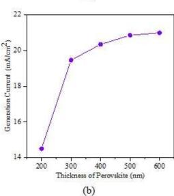
Fig. 4. Effect of absorber thickness on (a) integrated absorptance and (b) generation current
