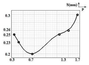
Fig. 7. Spot beam size (S) of the AiB with OV for the powers of the fractional FT (p).
