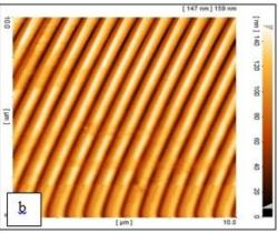
Fig. 1. The AFM image of 1D patterned PDMS fabricated using polycarbonate mold.
