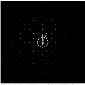
**Fig. 2.** Reciprocal lattice of 2-D 8-fold photonic quasicrystal, the first pseudo-Brillouin zone is indicated by white octagon
