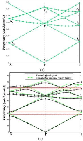
**Fig. 4.** (a) Band structure of unperturbed structure (empty lattice). (b) Band structure of considered 2-D 8-fold PQC (solid line) and the empty lattice (dashed line).
