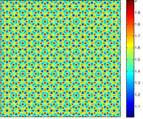
**Fig. 1.** Schematic representation of the top view of a pillar-type 8-fold PQC is illustrated. The rods indices of refractions vary in a 2D-quasi-periodic manner. The geometrical and physical parameters of the structure are given in Table I.
