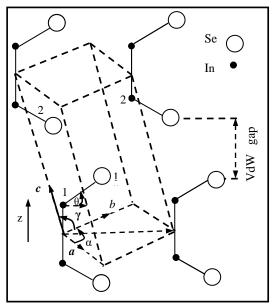
Fig. 1. Unit cell representation of  $\gamma$ -InSe. In the trigonal representation a=b=0.4002 nm, c=0.875 nm,  $\alpha=30^\circ$ ,  $\gamma=105^\circ$  and  $\theta=29^\circ$ . The main atoms' distances are In-In=0.282 nm, Se-Se=0.386 nm. The van der Waals gap width is 0.305 nm.
