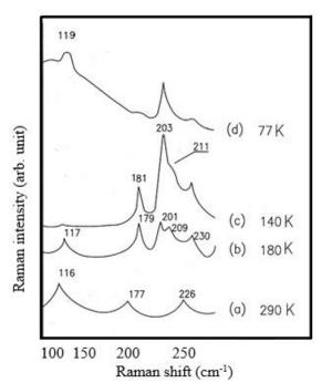
Fig. 2. One-phonon Raman spectrum of InSe at different temperatures recorded with excitation energy 2.54 eV of an argon ion laser. Spectrum (d) is compressed by 100 in order to bring it in proportionality to the other spectra.
