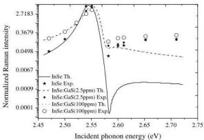
Fig. 4. Resonance curves for the 116 cm<sup>-1</sup> nonpolar mode at 20 K for InSe and various InSe:GaS doping densities. The Raman intensity is normalized with respect to 520 cm<sup>-1</sup> line of silicon and corrected for absorption. Solid lines are the curves obtained using Eq. (2) Ref.18, the discrete points are experimental points for InSe and InSe doped with GaS (2.5 ppm) and (100 ppm).
