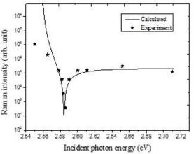
Fig. 3. Raman scattering cross section for  $A_{lg}^{l}$  optical phonon mode in InSe as a function of excitation energy at 20 K. The solid line is the theoretical calculation using Eq. (2) with  $E_g = 2.558 \text{ eV}$ .
