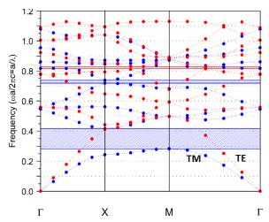
Fig. 1. The band structure of the fundamental PhC.
