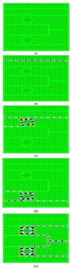
Fig. 5. The working states of the proposed encoder, (a) $I_0$ = $I_1$ = $I_2$ = $I_3$ =0, (b)  $I_0$ =1 and  $I_1$ = $I_2$ = $I_3$ =0, (c)  $I_1$ =1 and  $I_0$ = $I_2$ = $I_3$ =0, (d)  $I_2$ =1 and  $I_0$ = $I_1$ = $I_3$ =0, (e)  $I_3$ =1 and  $I_0$ = $I_1$ = $I_2$ =0.
