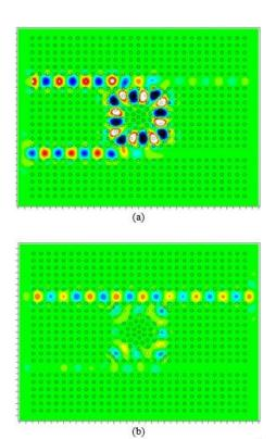
Fig. 3. Distribution of optical waves inside the structure for (a) Low and (b) High input optical power intensities.
