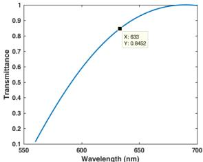
Fig. 4. The transmittance spectrum of dielectric-graphene photonic crystal.
