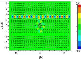
Fig. 4. The calculated electric field distribution inside the structure at two wavelengths (a) 1550 nm, and (b) 1560 nm.
