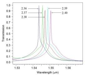
Fig. 9. The output spectra for different values of  $n_b$  and  $n_v$ .
