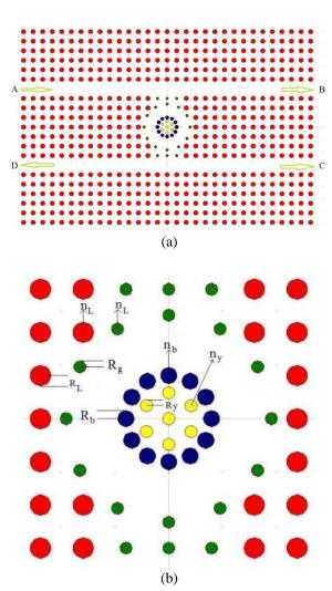
Fig. 2. (a) The schematic diagram of the proposed filter, (b) a macroscopic view of the resonant ring.
