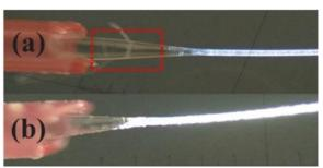
Fig. 1. Microscope image of (a) bare optical fiber etched to 28  $\mu m$  in diameter, (b) ZnO coated fiber with same diameter.
