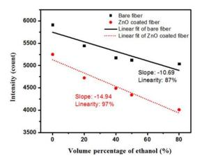
Fig. 6. Output intensity variation against ethanol concentration.
