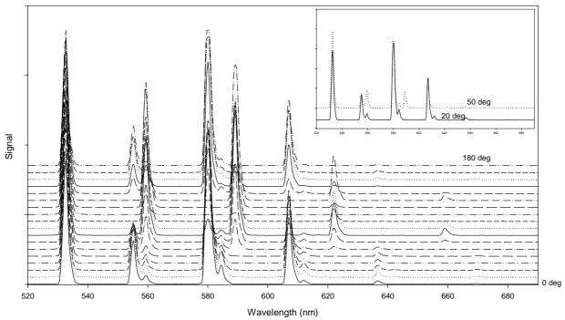
Fig. 7 Visible output spectra of the Raman laser as a function of the rotation angle f about the propagation axis. The rotation angle  $\phi=0$  deg corresponds to crystal aligned perpendicularly to the a-axis.
