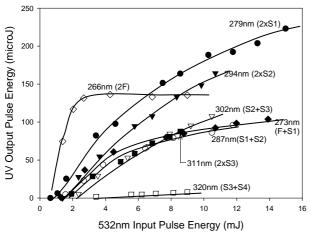
Fig. 4 Output energy at  $10 \, \text{Hz}$  for each UV wavelength as a function of input energy. (F = fundamental,  $S_n = \text{nth Stokes.}$ ).
