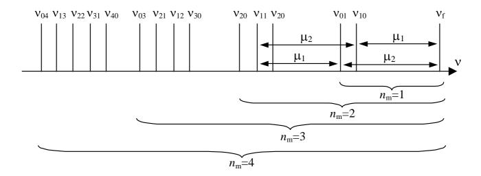
Fig. 6 Stokes spectra for Raman lasers with 1 and 2 active Raman modes shown for  $n_m \le 4$ .
