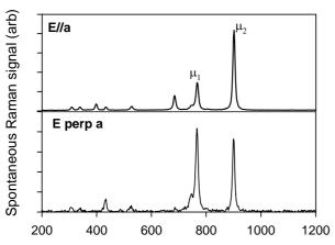
Fig. 5 Spontaneous Raman spectra for KGW for pump propagation along the  $N_{\rm p}$  axis and polarization aligned parallel and perpendicular to the crystal a-axis. Two strong Raman modes are observed at  $h\mu_1 = 768 cm^{-1}$  and  $h\mu_2 = 901 cm^{-1}$ .
