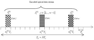
Fig. 7 Encoded pulses of 2-D optical CDMA system
