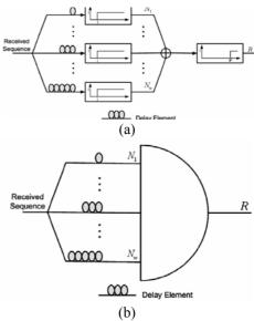
Fig. 4 (a) Ideal optical AND logic gate receiver structure for alloptical code recognition. (b) Equivalent functional AND logic gate receiver structure.
