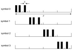
Fig. 5 An example of the transmitted signal formats of a single user in a PPM-CDMA system with M = 4, L = 8, and w = 3.
