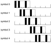
Fig. 6 An example of the transmitted signal formats of single user in an OPPM-CDMA system with M = 5, L = 9, and w = 3.
