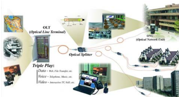
Fig. 12 Fiber-To-The-Home (FTTH) architecture and services
