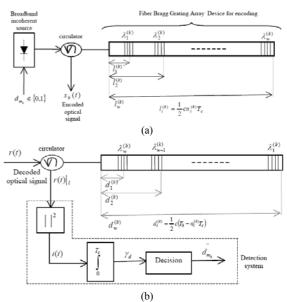
${\bf Fig.~8}$  (a) Encoding and (b) decoding structure based on FBG arrays.
