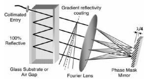
Fig. 10 Virtually Imaged Phased Array (VIPA) setup
