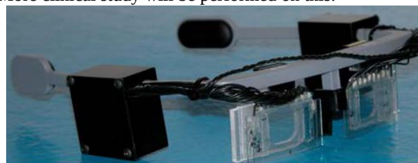
Fig. 11 A prototype of the assembled adaptive eyewear.
