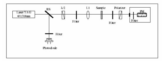
Fig. 1 Experimental setup for SHG measurements
