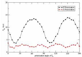
**Fig. 3** SHG intensity (arbitrary units) as a function of the fundamental beam polarization angle. Signal was detected with s (squares) and p (circles) polarizations. Incidence angle  $\theta$  was set at  $60^{\circ}$
