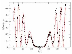
**Fig. 4**: SHG intensity (arbitrary units) as a function of the fundamental beam incidence angle from a glass slide having 7 bi-layers. Both laser and signal polarizations were set to p. The continuous curve is the theoretical fit of the data
