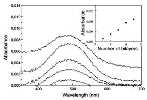
**Fig. 2** UV spectra of the (PAH/M-DR1) multilayer films. The curves from bottom to top are corresponding to the spectra of 1, 2, 3, 4 and 5 bi-layers. Inset shows the dependence of the absorbance on the number of deposited layers.
