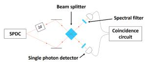
Fig. 3. The HOM interferometer
