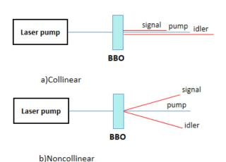
Fig. 1. (a) Collinear and (b) noncollinear geometries of SPDC procedure.
