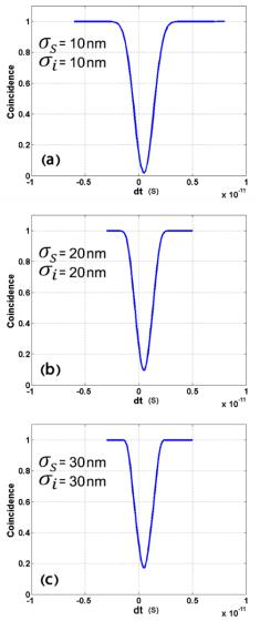
Fig. 7. The HOM dip plot for photon pairs generated by the SPDC for three different bandwidths of spectral filters.
