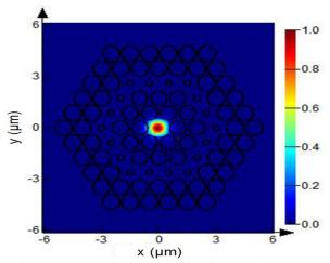
Fig. 3. The mode field distribution of the simple fiber at the wavelength of 1.55  $\mu m.$
