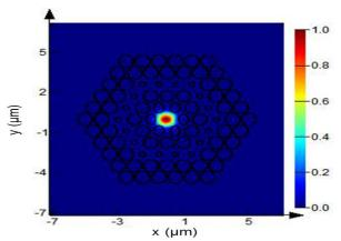
Fig. 6. The mode field distribution of the proposed fiber at the wavelength of 1.55  $\mu m$ .
