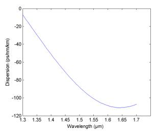
Fig. 12. The curve of dispersion compensating fiber with fluorine-doped silica rods.
