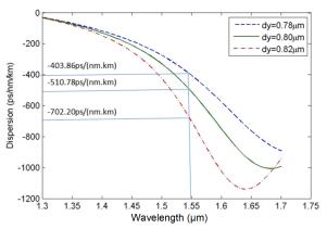
Fig. 9. The influence of the variation of the diameter of elliptical holes in the Y direction on the dispersion profile of the proposed fiber.
