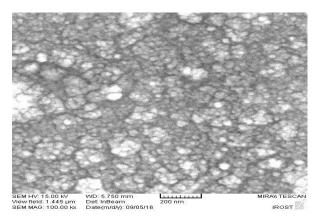
Fig. 9. The FESEM of NCD thin film from 15 to 50 nm grain sizes and ballast like on the CrN coated stainless steel, sample 3.
