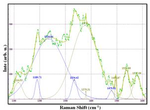
Fig. 11. Micro-Raman spectrum of the NCD film sample 3. The fitting has shown two shoulders at 1149 cm<sup>-1</sup> and 1471 cm<sup>-1</sup> as the sign of NCD film.
