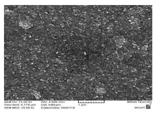
Fig. 10. The FESEM of NCD thin film from 50 to 150 nm grain sizes on the CrN coated stainless steel, sample 4.
