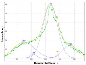
Fig. 12. Micro-Raman spectrum of the NCD film sample 4. The fitting has shown two shoulders at 1149 cm<sup>-1</sup> and 1471 cm<sup>-1</sup> as the sign of NCD film.
