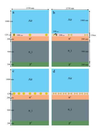
Fig. 3. Solar cell proposed structures Manipulated with: a, c) Spherical NPs with radius 50 nm; b, d) Tri-angular NPs
