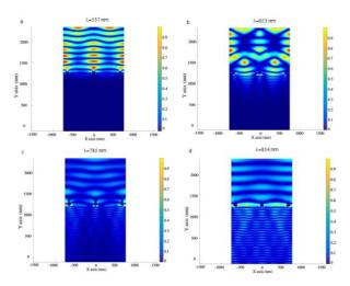
Fig. 7. Spherical NPs plasmonic effect on propagation of light in solar cell structure: a) 537 nm, b) 653 nm, c) 785 nm, and d) 854 nm.
