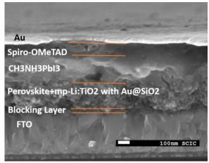
Fig. 3. The cross sectional SEM image of FTO/ bl-TiO<sub>2</sub>/ Au@SiO<sub>2</sub>/ mp-TiO<sub>2</sub>/ CH<sub>3</sub>NH<sub>3</sub>PbI<sub>3</sub>/ Spiro/ Au.
