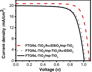
Fig. 5. The J–V curves of the cells consisting FTO/bl- TiO<sub>2</sub>/ Au@SiO<sub>2</sub>/ mp-TiO<sub>2</sub>/; FTO/bl- TiO<sub>2</sub>/ mp-
