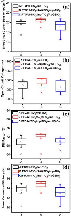
Fig. 7. Statistics parameters for the photovoltaic performance for 20 cells using different concentration of  $Au@SiO_2$  (a)  $J_{SC}$ , (b)  $V_{OC}$ , (c) FF, (d) PCE. A:FTO/bl-TiO<sub>2</sub>/mp-TiO<sub>2</sub>, B:FTO/bl-TiO<sub>2</sub>/Au@SiO<sub>2</sub>/ mp- TiO<sub>2</sub>, C:FTO/bl-TiO<sub>2</sub>/mp-TiO<sub>2</sub>/Au@SiO<sub>2</sub>.
