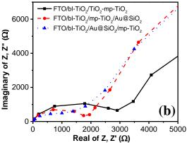
Fig. 9. The EIS using 0.2 V as applied DC voltage for sample without NP (FTO/bl-TiO<sub>2</sub>/ mp-TiO<sub>2</sub>) and with difference deposition place NPs (FTO/bl-TiO<sub>2</sub>/Au@SiO<sub>2</sub>/mp-TiO<sub>2</sub> and FTO/bl-TiO<sub>2</sub>/ mp-TiO<sub>2</sub>/Au@SiO<sub>2</sub>) (a) complete spectra; (b) zoom of different region of the complete plot.
