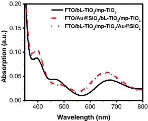
Fig. 4. Absorbance spectra of  $\overline{FTO}/$  bl-  $TiO_2/$  Au@SiO<sub>2</sub>/ mp-TiO<sub>2</sub>/;  $\overline{FTO}/$  bl-  $TiO_2/$  mp-TiO<sub>2</sub>/ Au@SiO<sub>2</sub> and the reference cells.
