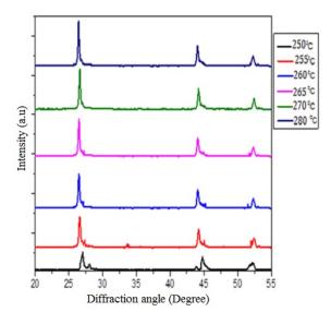
Fig. 2. Variation of CuIn0.5Ga0.5Se<sub>2</sub> diffraction peaks at different temperatures for 1.5 hour.
