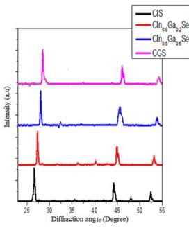
Fig. 1. Cu ( $In_xGa_{1-x}$ )  $Se_2$  XRD patterns for different x values, by heating-up method and for 1.5 hour procedure.
