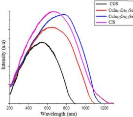
Fig. 5. CIGS absorption spectra for CGS, CuIn0.5Ga0.5Se<sub>2</sub>, CuIn0.8Ga0.2Se<sub>2</sub> and CIS nanoparticles.
