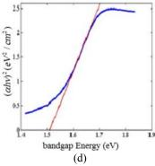
Fig. 6. The band gap energy of CIGS nanoparticles, calculated by Tauc equation, (a) CIS, (b) CuIn0.8Ga0.2Se<sub>2</sub>, (C) CuIn0.5Ga0.5Se<sub>2</sub>, (d) CGS.
