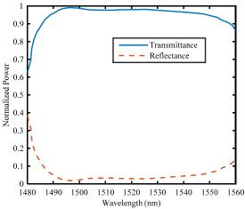
Fig. 5. The normalized transmission (summation of two output arms) and reflection for the proposed Y-splitter derived by FDTD method.
