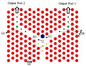
Fig. 2. The proposed Y-shaped photonic crystal topology for TE polarized incident light. The lattice defects have a radius equal to 0.3a, while the radii of the labeled holes are:  $r_a$ =0.12a,  $r_b$ =0.31a,  $r_c$ =0.4a,  $r_e$ =0.19a, and  $r_d$ =0.11a.
