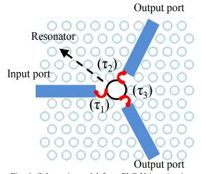
Fig. 6: Schematic model for a PhC Y-junction in a hexagonal lattice of circular holes embedded in a dielectric substrate. The radius of holes are equal to 0.3a.
