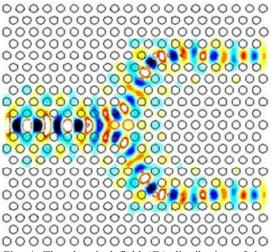
Fig. 4. The electrical field  $(E_Y)$  distribution of the power splitter topology depicted in Fig. 2. The input light wavelength is 1550nm.
