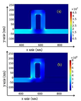
Fig. 5. Energy density inside the waveguide shown in Fig. 1(b) where w=50 nm, d=100 nm, h=200 nm,  $w_d=100$  nm, and  $w_s=50$  nm for the wavelengths: (a)  $\lambda = 610$  nm, and (b)  $\lambda = 738$  nm.
