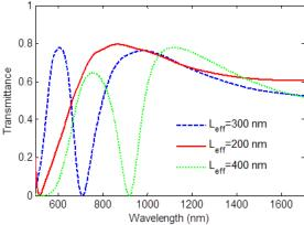
Fig. 6. Transmittance spectra of the waveguide shown in Fig. 1(a) for  $L_{eff}$  =200 nm,  $L_{eff}$  =300 nm, and  $L_{eff}$  =400 nm, where d=100 nm, w=50 nm, and w<sub>s</sub>=50 nm.
