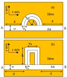
Fig. 1. Structural geometry of an MIM waveguide containing, (a) a semi-circular and (b) rectangular ring shaped groove.
