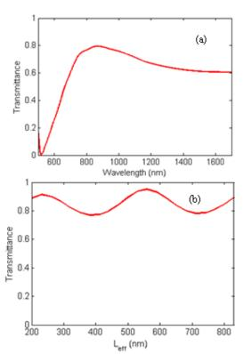
Fig. 2. (a) Transmittance spectrum of the waveguide shown in Fig. 1(a) where w=50 nm, d=100 nm,  $L_{eff}$ =200 nm, and  $w_s$ =50 nm; (b) transmittance of the semi-circular ring shaped groove itself as a function of  $L_{eff}$  at  $\lambda$  = 868 nm.
