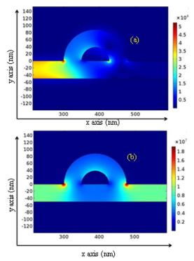
Fig. 4. Energy density inside the waveguide shown in Fig. 1(a) where  $L_{eff}$  =200 nm, w=50 nm, d=100 nm, and w<sub>s</sub>=50 nm for the wavelengths: (a)  $\lambda$  = 519 nm, and (b)  $\lambda$  = 868 nm.
