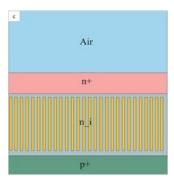
Fig. 1. Solar cell structures (a) without any NPs (traditional), (b) with NPs in the addition region, and (c) NRs in the intrinsic area"
