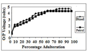
Fig. 8. Experimental results for petrol and diesel adulteration percentage using optical fiber sensor
