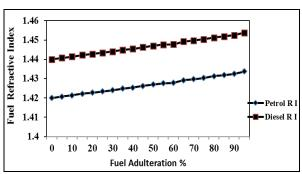
Fig. 7. Measured refractive index of adultrated fuel using Abee's Refractometer.
