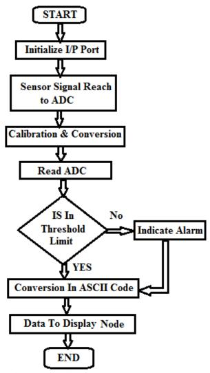
Fig. 6. Flow chart for real time process model to display adulteration level using PIC.
