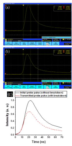
Fig. 2. (a) Initial probe signal when the pump laser beam is blocked, (b) Transmitted probe beam when the optical breakdown plasma induced (in colloidal TiO<sub>2</sub> nanoparticles) at 46.0 GW/cm<sup>2</sup> pump laser intensity, and (c) Comparison of signals (a) and (b).
