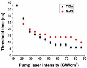
Fig. 5. Threshold time versus pump laser intensity for laser induced breakdown for NaCl in distilled water (circles) and in colloidal TiO<sub>2</sub> nanoparticles (squares).
