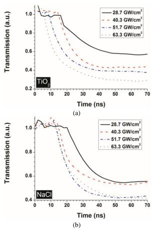
Fig. 3. Time-resolved transmission of the probe beam through the breakdown plasma at 28.7, 40.3, 51.7, and 63.3 GW/cm<sup>2</sup> pump laser intensities for TiO<sub>2</sub> nanoparticle and NaCl in distilled water.
