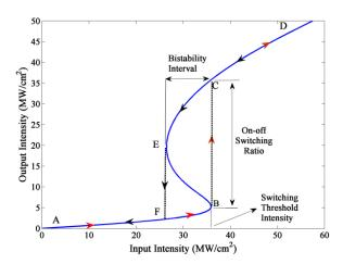
Fig. 2. Typical optical bistability diagram.
