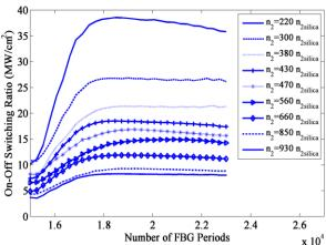
Fig. 9. The on-off switching ratio versus number of FBG periods for nine chalcogenide glassess of different third order refractive indicies.
