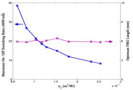
Fig. 10. The maximum on-off switching ratio and optimum FBG length versus third order refractive index of chalcogenide glassess.
