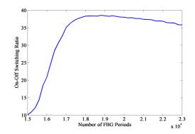
Fig. 6. The on-off switching ratio as a function of number of FBG periods.
