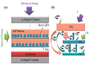
Fig. 1 (a) The schematic of 1.55µm QD laser structure (b) Carrier transition times. An excess number of carriers are provided to the ES through absorption of the external optical pump [20].
