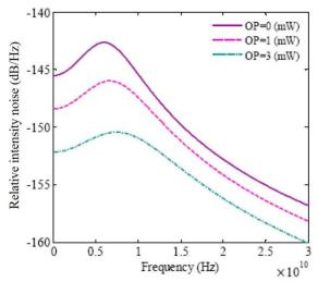
Fig. 8 The relative intensity noise spectrum of InAs/InP QD laser for three different values of optical pumping and at the injection current of *I*=55mA. External optical beam decreases the level of RIN and increases the damping factor.
