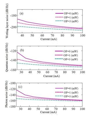
Fig. 9 The values of the (a) WL, (b) quantum, and (c) photon noises versus current at f=1GHz for three different optical pump powers. External optical beam reduces the values of three shot noise sources at all bias points.
