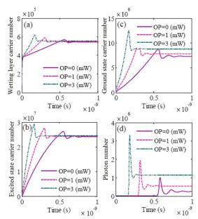
Fig. 6 Turn-on dynamics of carriers and photons for a step current from zero to I=55mA. The number of carriers at all three states of the (a) WL, (b) ES, and (c) GS and also (d) photons grow during shorter delay time by increasing the external optical pump.
