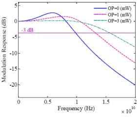
Fig. 4 Modulation response of QD laser for three different values of optical pumping and at *I*=55mA. Optical pump makes the modulation response of QD laser wider and increases its 3dB bandwidth.
