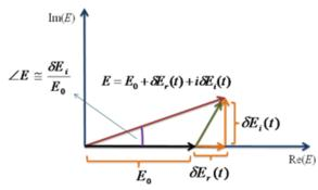
Fig. 2 Vector illustration of the relationship between the instantaneous field magnitude and the in-phase and out-phase noise components [25].
