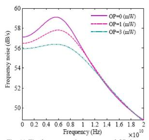
Fig. 11 The frequency noise spectrum of QD laser for three different optical pump powers and at the injection current of I=55mA. The FN level reduces and the resonant frequency grows at higher optical pumps.
