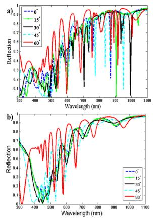
Fig. 3 Simulated reflection spectra in a) c-Si nanobar structure b) B-structure at various angles of incidence.
