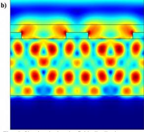
Fig. 5 Simulated electric field distribution at an operating wavelength of a) 530nm, b) 760nm.
