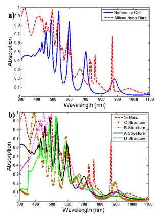
Fig. 4 a) Simulated optical absorption spectra of a c-Si thin film solar cell with (red dashed line) and without (solid blue line) c-Si nano-bars anti-reflection coating. b) Simulated optical absorption spectra of a c-Si thin-film solar cell with different AR coatings.
