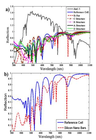
Fig. 2. (a) Simulated reflection spectra of the structure with (red dashed line) and without (solid blue line) nano-bars versus wavelength. (b) Reflection spectra of all five structures as introduced in Table 1 together with the reference cell and the AM1.5G solar spectrum.
