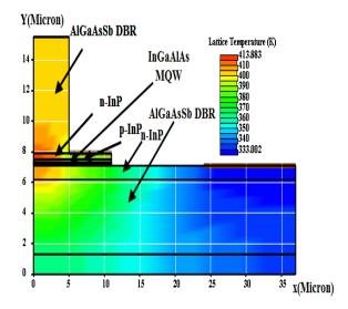
Fig. 4: Two- dimensional temperature distribution of laser with 10 nm electron stopper layer thickness at maximum power for 60 °C stage temperature.
