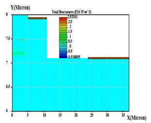
Fig. 14: Two- dimensional heat power distribution of laser with 10 nm electron stopper layer offset at maximum power for  $60\,^{\circ}\text{C}$  stage temperature.
