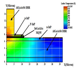
Fig. 15: Two- dimensional temperature distribution of laser with 20 nm electron stopper layer thickness and with  $5\times10^{23}$  cm<sup>-3</sup>p- doping level at maximum power for 60 °C stage temperature.
