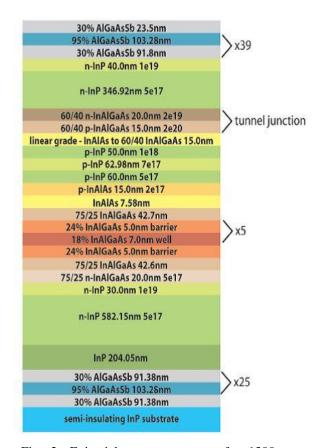
Fig. 2: Epitaxial structure grown for 1300 nm VCSELs.
