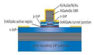
Fig. 1: Schematic of a 1.3  $\mu$ m VCSEL structure.
