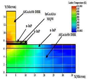
Fig. 16: Two- dimensional temperature distribution of laser with 20 nm electron stopper layer thickness and with  $7 \times 10^{23}$  cm<sup>-3</sup>p- doping level at maximum power for 60 °C stage temperature.
