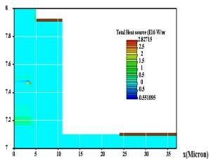
Fig. 8: Two- dimensional heat power distribution of laser with 10 nm electron stopper layer thickness at maximum power for 60 °C stage temperature.
