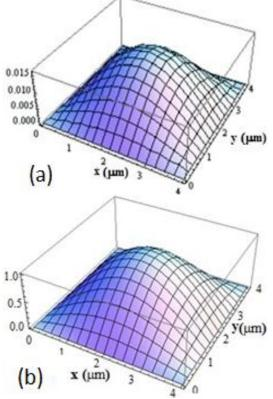
Fig. 5. The electric field distribution for the fundamental mode of the rectangular waveguide at  $\beta_1$ =15.55 found (a) numerically and (b) analytically. Vertical coordinate is the relative Electric Field amplitude.
