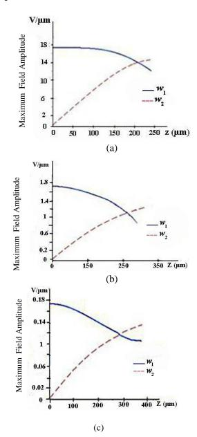
**Fig. 7**. The evolution of maximum amplitude along the fiber for the initial signal of (a)  $1000\Phi_0$ , (b)  $100\Phi_0$ , and (c)  $10\Phi_0$  at z=0, where  $w_1$  and  $w_2$  are the field amplitudes of input signal and the generated second harmonic, respectively.
