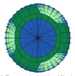
Fig. 2. The cross sectional meshing of fiber shown in Fig. 1 emphasizing the core's mesh.
