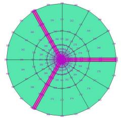
Fig. 1. A typical mesh for wagon wheel fiber's cross sectional view.
