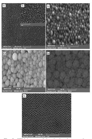
Fig. 2. SEM images of the cicada wing top view  $(C_0)$  and tilted view  $(C_1)$  showing the structures of nanonipple arrays; the surface structures of the Ag nanostructures obtained in different operational conditions of dc magnetron sputtering  $(C_2, C_3,$  and  $C_4)$ ; the back side of nanocauliflower arrays, the structure of quasi-ordered nano-hole arrays  $(C_5)$  imprinted from nanonipple arrays onto the silver deposited layer.
