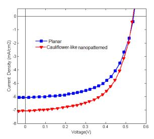
Fig. 5. Current density-voltage (J-V) characteristics of the planar and cauliflower-like nanopatterned back electrode devices measured under AM 1.5 illuminations at 100 mW/cm<sup>2</sup>
