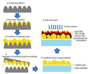
Fig. 1. Schematic diagram of the fabrication procedure of OSC with cauliflower-like nanostructure arrays, using the cicada wing as a biotemplate. The specification of the fabricating steps (a)–(e) for the back electrode layer and (f) for the spin-coated layers and semitransparent metal electrode (STME) deposited on the solar cell in the scheme.
