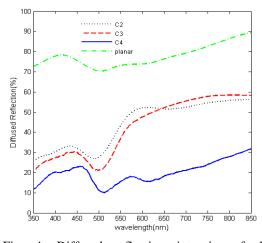
Fig. 4. Diffused reflection intensity of three nanostructure samples ( $C_2$ ,  $C_3$ , and  $C_4$  compared with the planar substrate) fabricated in different operational conditions of magnetron sputtering vs. incident light wavelength.
