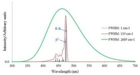
Fig. 10. Computed absorption spectrum of solvated DCM by including the vibrational couplings during electronic excitation. Different full width at half maximum (FWHM) have been chosen in convoluting gaussian (red, green and blue stick line).
