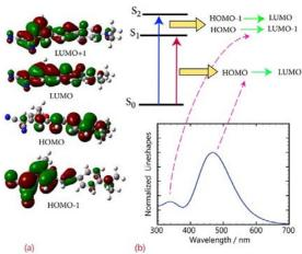
Fig. 6. (a) Canonical Orbitals which is included in first two singlet electronic excitation processes. (b), Computed absorption spectrum of solvated DCM resulted from vertical excitation computation without vibrational couplings. Schematic diagram depicts each of transition processes. All computation have been performed at PCM-TD-B3LYP/6-31G(d) level.
