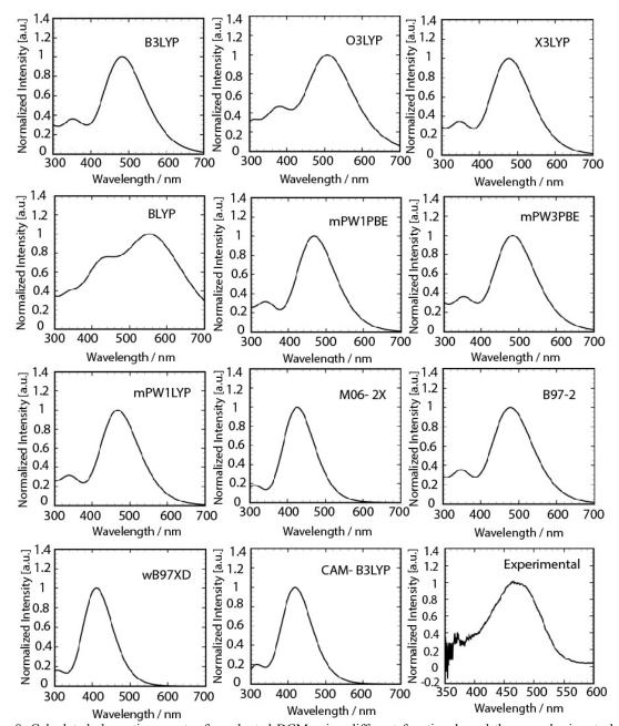
Fig. 8. Calculated absorption spectra for solvated DCM using different functionals and the same basis set along with experimental spectra.
