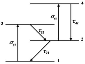
Fig. 1. The four-level model of the saturable dye.
