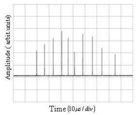
**Fig. 7.** Oscillogram of a train of output pulses,  $T_0 = 59.3\%$  and pulse pump energy 41J.
