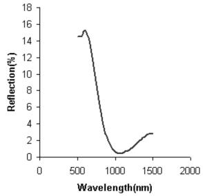
Fig. 3. The coated BK7 glass reflection spectrum.
