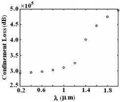
**Fig. 6**. Confinement losses spectrum for  $d/\Lambda=0.8$ .
