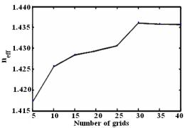
**Fig. 3**. Variation of effective refractive index vs. grid numbers.
