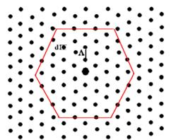
Fig. 2. PCF with a hexagonally-packed rings of holes
