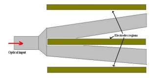
**Fig. 3** Application of electrode region in the Y-branched DOS.
