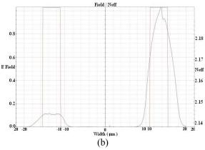
**Fig. 7** Operation at  $1.55 \mu m$  optical powers input with -24 V bias on middle electrode. (a) Optical field propagation in the DOS architecture (b) cut view of the output section, graph showing electric field intensity (curved shaped) and refractive index distribution (rectangular shaped) over the section.
