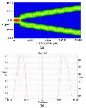
**Fig. 4** Operation at 1.55 μm optical power input (a) Optical Field propagation in the DOS architecture (b) cut view of the output section, graph showing electric field intensity (curved shaped) and refractive index distribution (rectangular shaped) over the section.
