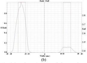
**Fig. 6** Operation at 1.55 μm optical powers input with +24 V bias on middle electrode. (a) Optical field propagation in the DOS architecture (b) cut view of the output section, graph showing electric field intensity (curved shaped) and refractive index distribution (rectangular shaped) over the section.
