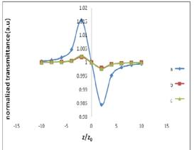
**Fig. 5** Normalized closed aperture Z-scan (S=0.4) of a) CdS direct band gap crystal and b) CdI<sub>2</sub>, c) PbI<sub>2</sub> indirect band gap crystals showing  $\Delta T_{p-\nu}$  at  $\lambda$ =532nm. The solid curves are the theoretical fit with experimental data.
