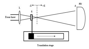
Fig. 1 Open aperture z-scan
