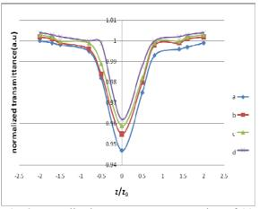
**Fig. 3** Normalized open aperture Z-scan data of (a) CdS (b) ZnS (c) ZnO (d) GaN (direct band gap crystals) measured with 7ns pulses at  $\lambda$ =532 nm. The solid curves are the theoretical fit with  $\tau$ =(1.3±0.6) ns.
