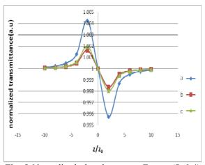
**Fig. 8** Normalized closed aperture Z-scan (S=0.4) of a) GaN direct band gap crystal and b) CdI<sub>2</sub>, c) PbI<sub>2</sub> indirect band gap crystals showing  $\Delta T_{p-\nu}$  at  $\lambda$ =532nm. The solid curves are the theoretical fit with experimental data.
