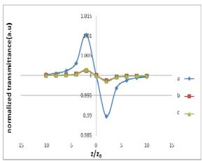
**Fig. 7** Normalized closed aperture Z-scan (S=0.4) of a) ZnO direct band gap crystal and b) CdI<sub>2</sub>, c) PbI<sub>2</sub> indirect band gap crystals showing  $\Delta T_{p-\nu}$  at  $\lambda$ =532nm. The solid curves are the theoretical fit with experimental data.
