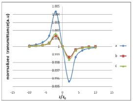
**Fig. 6** Normalized closed aperture Z-scan (S=0.4) of a) ZnS direct band gap crystal and b) CdI<sub>2</sub>, c) PbI<sub>2</sub> indirect band gap crystals showing  $\Delta T_{p-v}$  at  $\lambda$ =532nm. The solid curves are the theoretical fit with experimental data.
