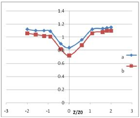
**Fig. 4** Normalized open aperture Z-scan data of a)  $CdI_2$  and b)  $PbI_2$  (indirect band gap crystals) measured with 7ns laser pulses at  $\lambda$ =532nm. The solid curves are the theoretical fit with  $\tau$ =(1.1±0.04) ps.
