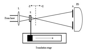
Fig. 2 Closed aperture z-scan
