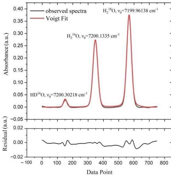
Fig. 3. Voigt Fit and residuals of absorption isotope peak of water.
