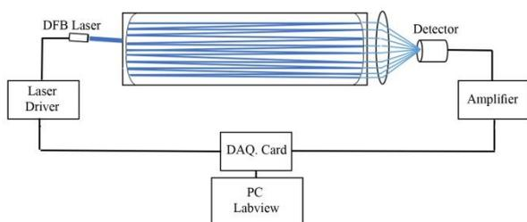
Fig. 1. Experimental setup of water isotope analyzer.
