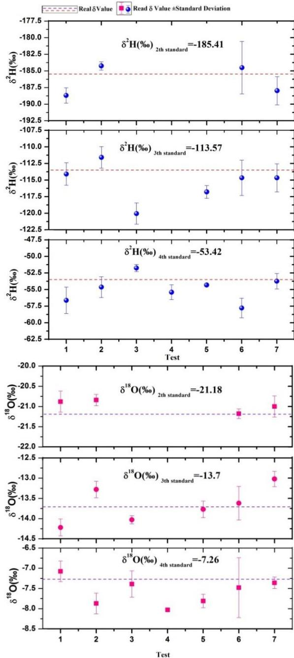
Fig. 7. The  $\delta^2H$  and  $\delta^{18}O$  results are related to the accuracy of the present laser system readings, which range from 4 to 7 across three different samples. The dashed line indicates the actual concentration of the samples, and the error bars on each result represent the measurement precision after five repetitions. The measurement precision is expressed as the  $\pm$  standard deviation of the results.
