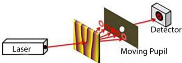
Fig. 4. Efficiency measurement of the diffraction order setup.
