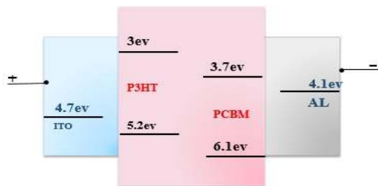
Fig. 4. The place of thin film, the electrodes and their energy levels.
