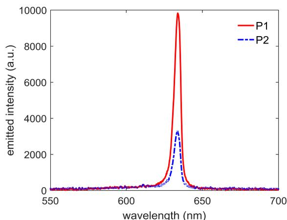
Fig. 5. Comparison between the emission spectra of S1 (sample 1) corresponding to the two different excitation positions P1 (position 1) and P2 (position 2) at the pump fluence 169.8 mJ/cm<sup>2</sup>.
