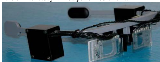
Fig. 11 A prototype of the assembled adaptive eyewear.
